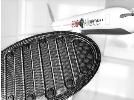
Figure 4 : Aeronautical component with overmolded inserts
